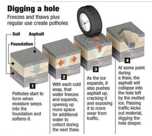
Road pavements suffer various deteriorations during their lifetime, which requires a lot of money to repair. One of the most common forms of these distresses is the pothole that affects the durability and life span of the pavement and repairing them costs millions of euros annually.
